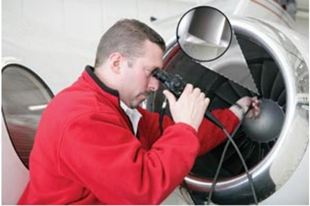
With their ability to see places where the unaided human eye can't, borescopes are incredibly valuable for aircraft maintenance technicians. But like all good tools, there are right ways and wrong ways to use borescopes; especially when it comes to nondestructive testing (NDT) of components and airframes.
