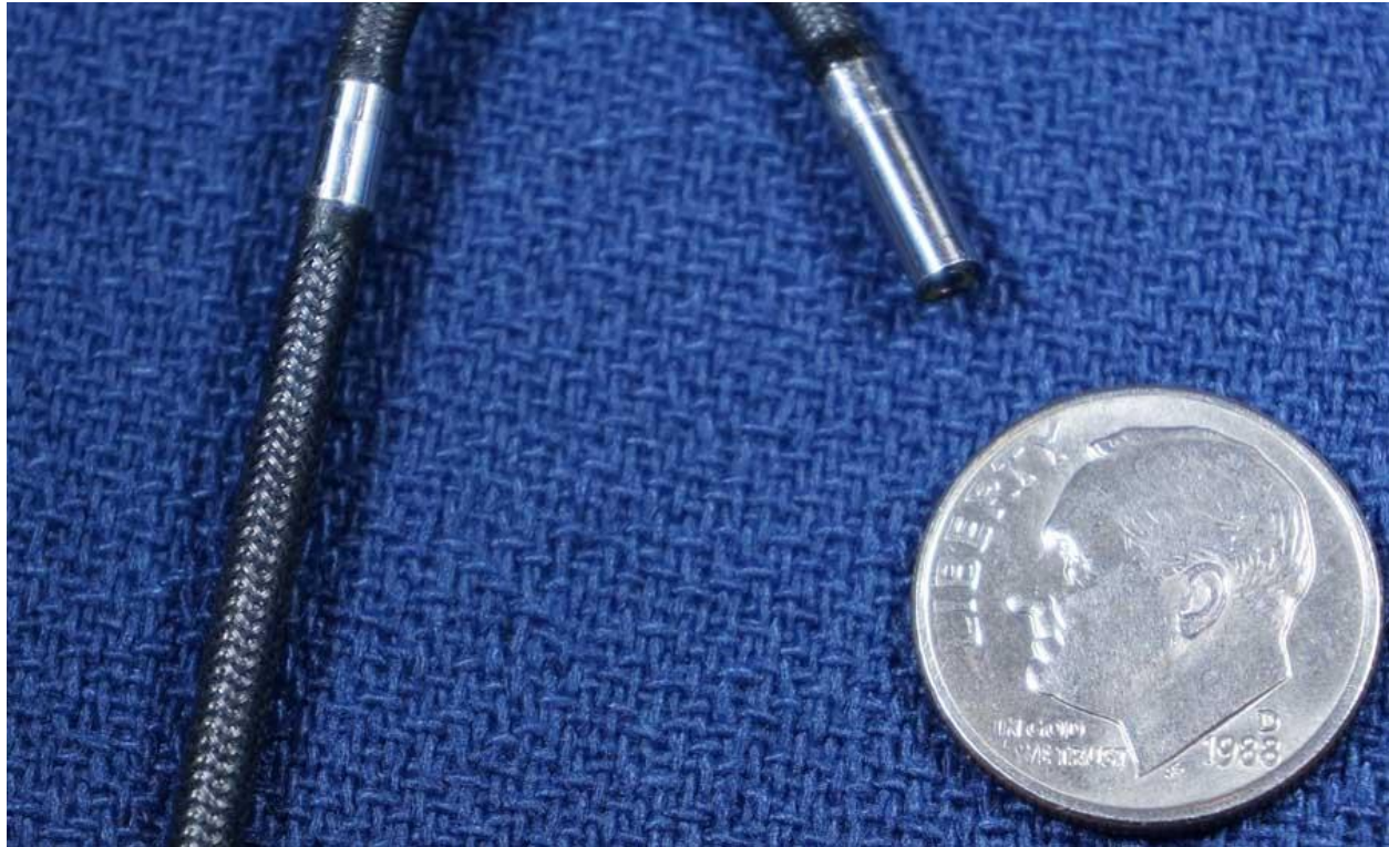
2.8mm insertion tube and dime
