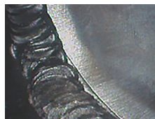
Pipe weld image taken using the VJ-3 articulating video borescope
